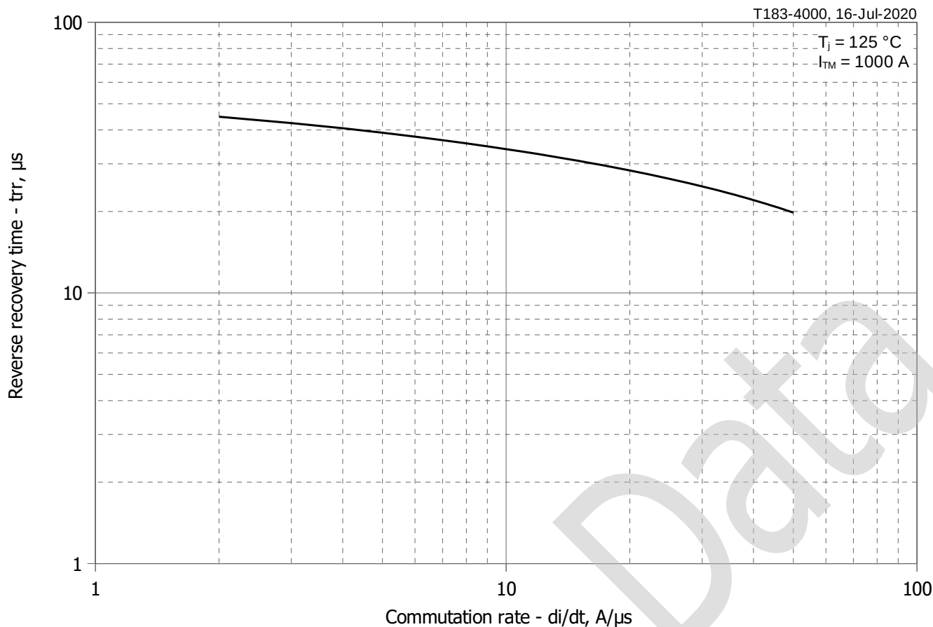
Fig. 5 – Maximum recovery time t_{rr} vs. commutation rate di_R/dt (25% chord)
