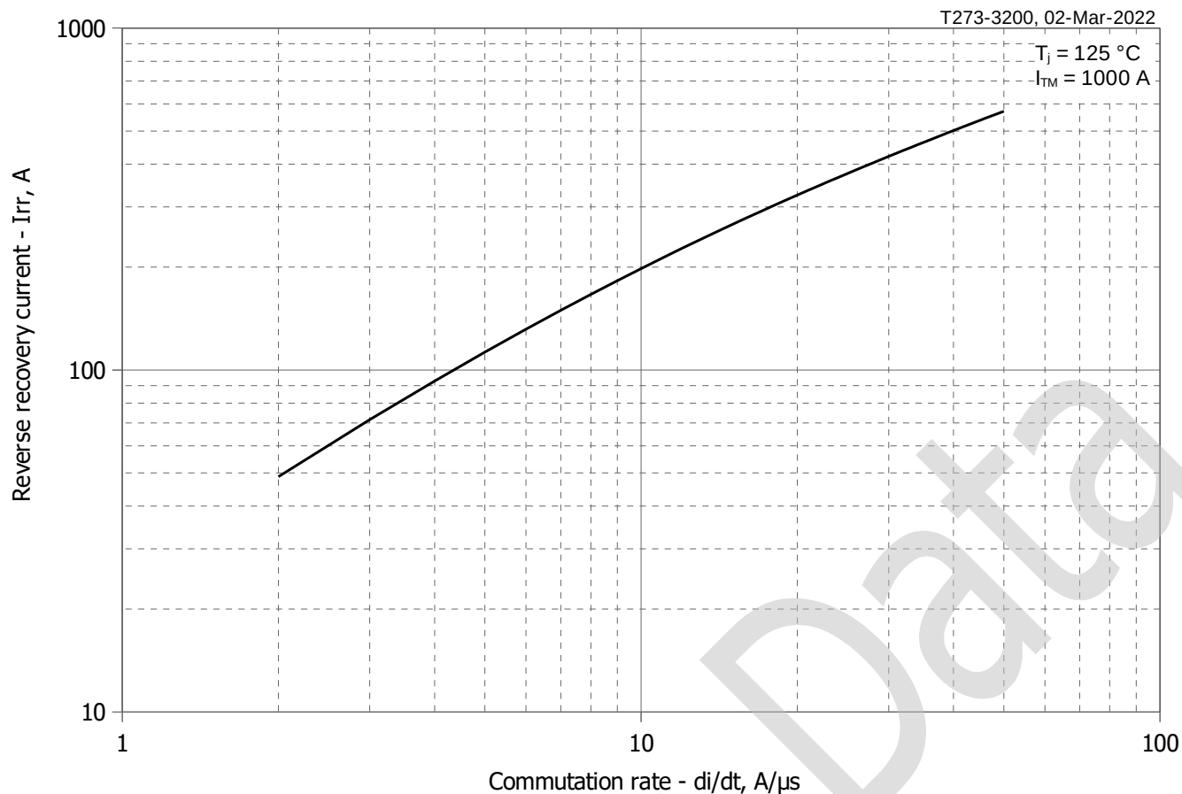
Fig 7 – Maximum reverse recovery current I_{rr} vs. commutation rate di_R/dt
